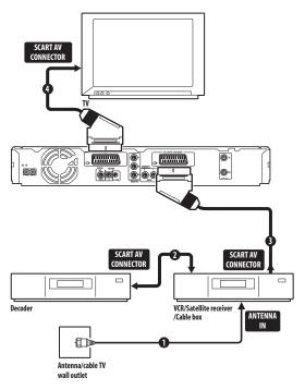
1 Connect the cable from the antenna/cable TV outlet to the antenna input on your VCR/satellite receiver/cable box.
